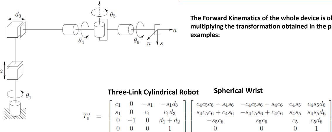
The Forward Kinematics of the whole device is obtained by multiplying the transformation obtained in the previous examples:
