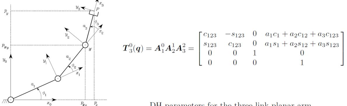
DH parameters for the three-link planar arm
