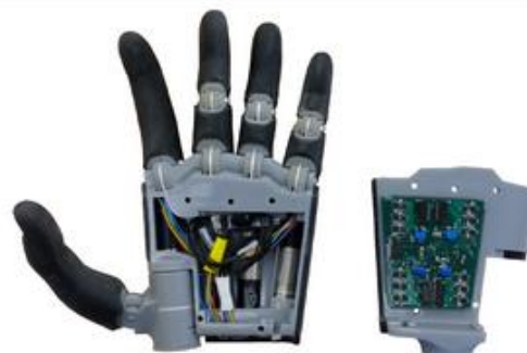
Assembled hand with cover removed: Left: bottom of hand with 4 brushless DC servomotors Right: top of hand with servoamplifier circuit board
