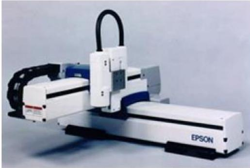
Figure 1.17: The Epson Cartesian Robot. Photo courtesy of Epson.
