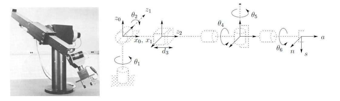
This manipulator is an example of a spherical (RRP) manipulator with a spherical wrist. This manipulator has an offset in the shoulder joint that slightly complicates both the forward and inverse kinematics problems.
