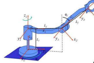
*The obtained transformation is the forward kinematics of the manipulator.*
