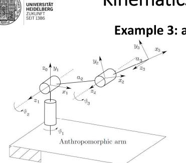
$$\mathbf{F}_{3}^{0}(\boldsymbol{q}) = \mathbf{A}_{1}^{0}\mathbf{A}_{2}^{1}\mathbf{A}_{3}^{2} = \begin{bmatrix} c_{1}c_{23} & -c_{1}s_{23} & s_{1} & c_{1}(a_{2}c_{2}+a_{3}c_{23}) \\ s_{1}c_{23} & -s_{1}s_{23} & -c_{1} & s_{1}(a_{2}c_{2}+a_{3}c_{23}) \\ s_{23} & c_{23} & 0 & a_{2}s_{2}+a_{3}s_{23} \\ 0 & 0 & 0 & 1 \end{bmatrix}$$
