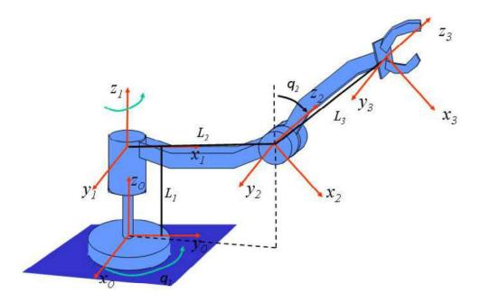
Knowing the *geometrical features* of a manipulator and associating to each link a *reference frame,* we are able to use *homogenous transformations* among the links and formulate the <u>Kinematics</u>
