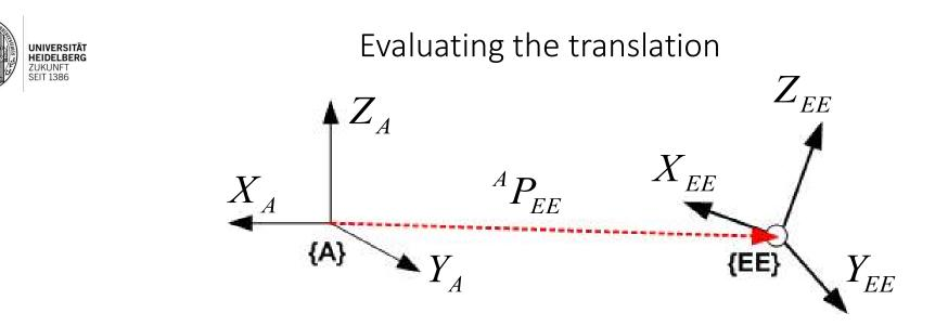
${}^{A}P_{EE}$  is the projection of the position of **{EE}** into the unit vectors of the frame **{A}**.
