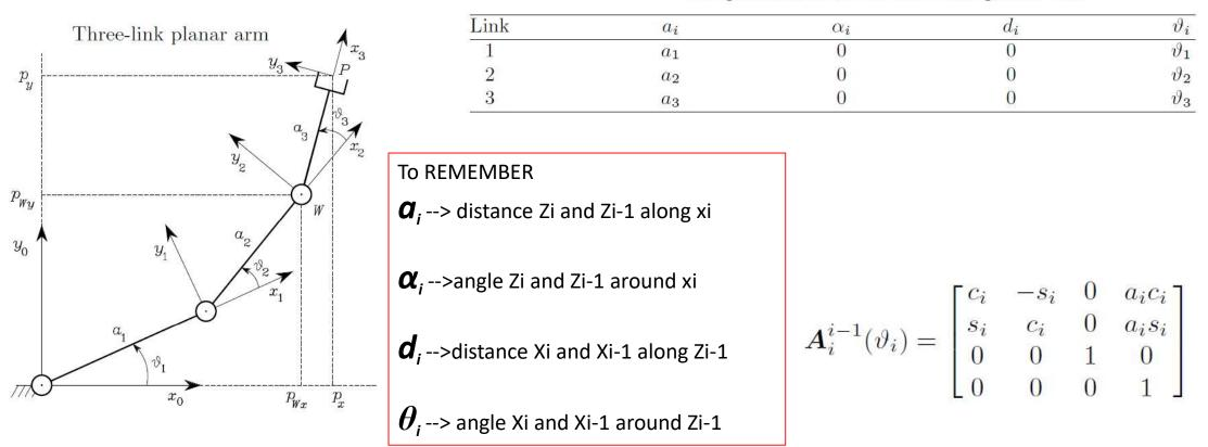
DH parameters for the three-link planar arm
