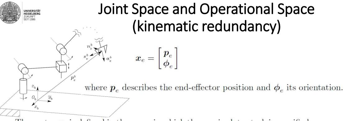
The vector  $\boldsymbol{x}_e$  is defined in the space in which the manipulator task is specified; hence, this space is typically called *operational space*.
