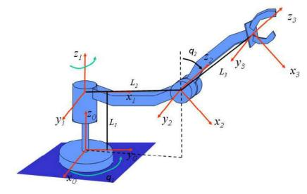
Considering the four frames, arbitrary chosen on the four links, it is possible to write down the matrixes of the single homogeneous transformations.
