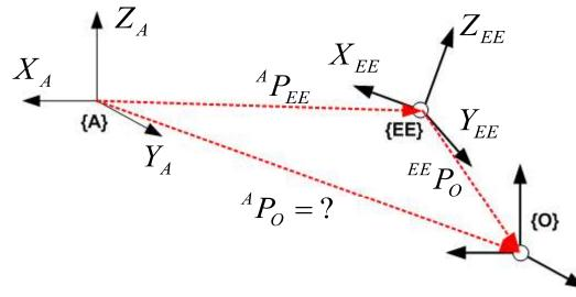
General case when we know the position of an object **{O}** in a frame **{EE}** and we want to know its position respect to the frame **{A}**
