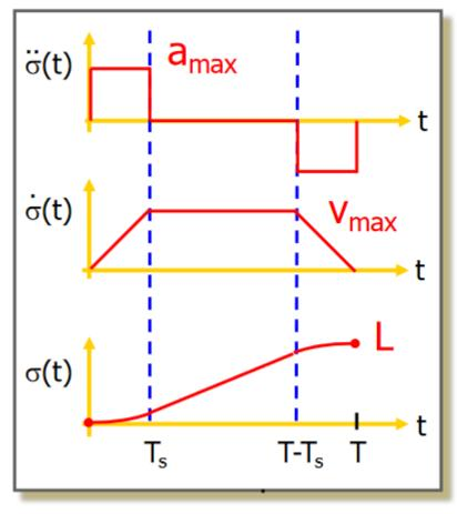
$$\sigma(t) = \begin{cases} a_{max} \ t^2/2 & t \in [0,T_s] \\ v_{max} \ t - \frac{v_{max}^2}{2 a_{max}} & t \in [T_s, T - T_s] \\ - a_{max} \ (t - T)^2/2 + v_{max} \ T - \frac{v_{max}^2}{a_{max}} \\ & t \in [T - T_s, T] \end{cases}$$
