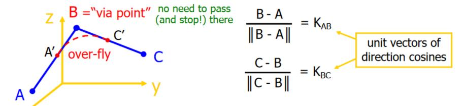
given: constant speeds  $v_1$  on linear path AB  $v_2$  on linear path BC
