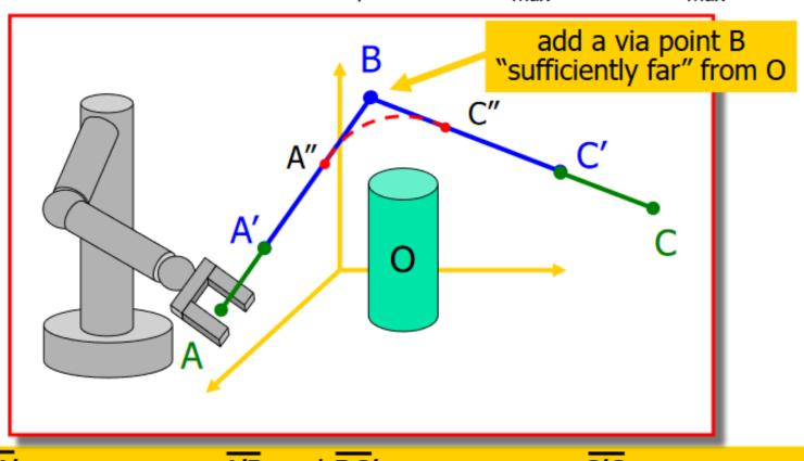
on  $\overline{AA'} \to a_{max}$  on  $\overline{A'B}$  and  $\overline{BC'} \to v_{max}$  on  $\overline{C'C} \to -a_{max}$  + over-fly between A" e C"
